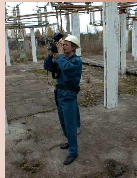
Technicians use a U.S.-supplied infrared thermography unit to detect hot spots in electrical systems before equipment fails.
