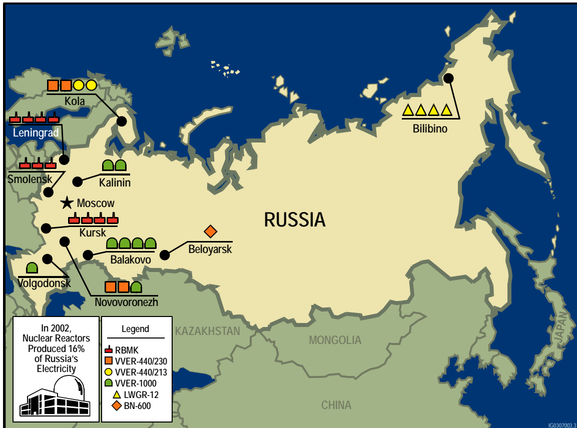
Figure 5. Nuclear Power Plants in Russia Participating in the U.S. Program to Improve Nuclear Safety
